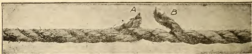
Fig. 1. A Broken Strand to Be Repaired.
